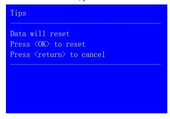
**Notice:** sometimes when users change output cards by themselves, the data of new output cards might be inconsistent with that saved by the system. "**Reset data**" will restore the data of new output cards to the factory default. The operation is only valid for a single output card, so it won't affect the data of other output cards.
