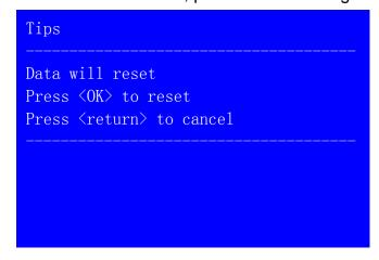
**Notice:** to change the output port will restore the data of the output card, don't change it if unnecessary.
