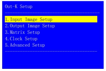
Press " ↑ , ↓ " to select the setting, turn the knob to ajust, and press "**OK**" to confirm.
