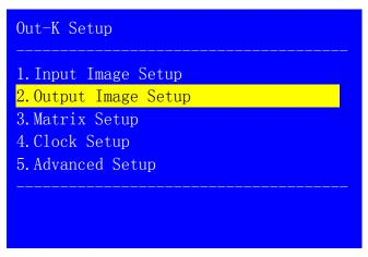
Press "↑, ↓" to select the setting,turn the Knob to ajust, and press "**OK**" to confirm.
