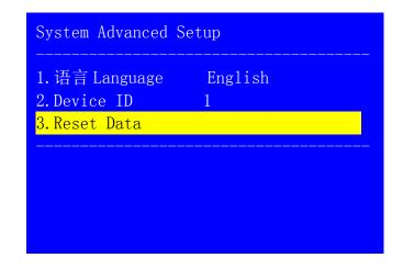
On the sub menu of "Reset Data", press "**OK"** to reset.
