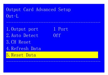
On the sub menu of "Reset Data", press "OK" to reset.
