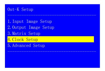
Press "↑, ↓ "to select the setting, turn the knob to ajust, press "**OK**" to confirm.
