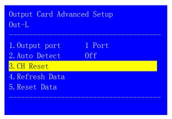
**Notice:** input signals for output cards will be briefly unstable when making changes in "Matrix K Setup" or "Matrix L Setup" and it will lead to blurred or blank screen. "**CH Reset**" will restore the system. Normally this operation is not necessary.
