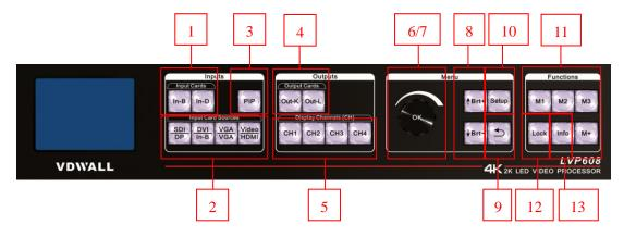
Input Cards (In-B, In-D): stand for 2 input cards accordingly. In-B is Full HD Video Input Card. In-D is Ultra HD Video Input Card. When pressing a button to select a card, if the red light of the indicator is on, it means the operation of the current input card is valid.
