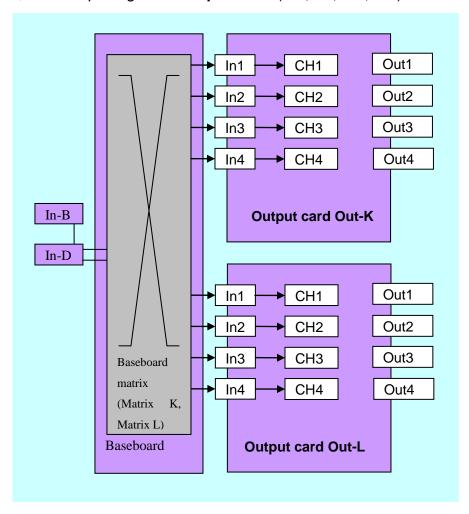
The **output card** design of **LVP608** has 3 different output modes. In this device, the design currently has: **four ports**, **two ports** (**up/down**) and **one port**, **c**ustomers can select output modes according to the project requirements.
