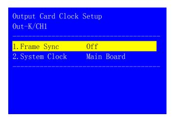
Notice: clock setup is only used when display is out of sync,if display is out of sync,please set "Frame Sync" as In1,and also select "System Clock"as In1.
