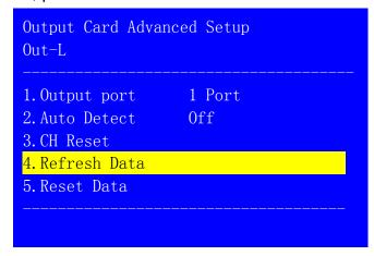
**Notice:** sometimes when users change output cards by themselves, the data of new output cards might be inconsistent with that of the system. "**Refresh Data**" will then update the system data to be consistent with that of the new output cards.
