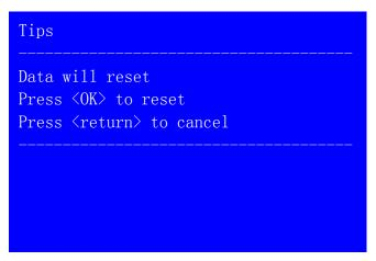
**Notice**: sometimes when users change input cards by themselves, the data of new input cards might be inconsistent with that saved by the system. "Reset data" will restore the data of new input cards to the factory default. The operation is only valid for a single input card, so it won't affect the data of other input cards.
