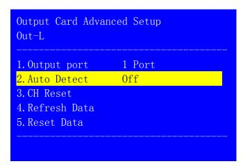
**Notice:** normally "Auto detect" is off, it is mainly used for malfunction detec of input card. When "Auto detect" is on and In-D has malfunction, the screen will be blank.
