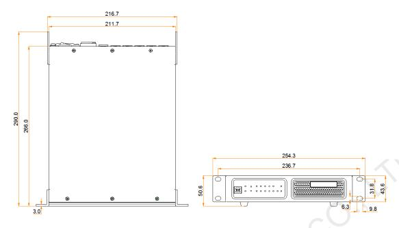
Tolerance: ±0.3 Unit: mm
